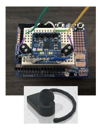
consists of an Arduino microcontroller, infrared thermometer, and 3D printed Arduino housing and earpiece. The infrared thermometer is located inside of the earpiece and focused on the tympanic membrane. The sensor sends the output to the Arduino via a wire, where the data are stored.
