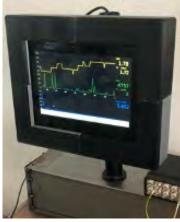
They then undergo a peak detection scheme to identify the QRS complex and systolic magnitude for the ECG and BP waveforms, respectively. This is then serially communicated to a Graphical User Interface (GUI) running on a Raspberry Pi that facilitates user interaction with the data. The GUI has various capabilities such as external data download, flagging and comment on specific data points, and trend analysis for the input HRV and BRG data.
