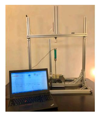
to replicate the magnitude and direction of impacts seen in surgical settings. Therefore, the project involved designing and building an impact test device that allows the client to test various types of implants with their respective inserters. The device can test a spinal cage and inserter at various angles and impact forces.
