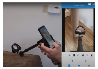
functionality. The final prototype consisted of telescoping tubing to obtain the correct focus and focal points for different diopter lenses, a fully rotatable lens mount to aid in removing flash reflections, a bike mount phone holder to securely hold the user's phone in place to take a picture, and a handle to hold the fixture.
