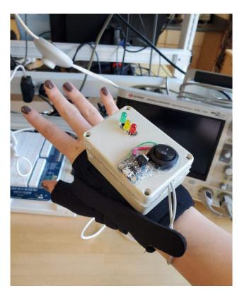
contracting the target muscle, no LEDs would light. A minor contraction would trigger the red LED, a moderate contraction would trigger the yellow LED, and a full correct contraction would trigger the green LED. The main device components include a compressive glove, electrodes, LEDs, pre-processing circuit (to read, amplify, and reduce signal noise), microcontroller (to queue the LEDs), and postprocessing circuit (the LEDs).
