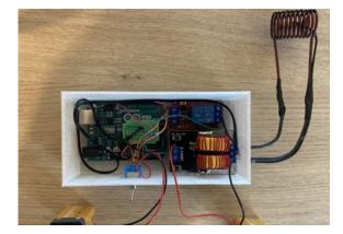
temperature gradient to reduce fogging of the lens. The purpose of this project was to develop a solution that would reduce the fogging of the lens without the need for the surgeon to remove, clean, and reinsert the scope. The device could not increase the diameter of the scope, and had to be as lightweight as possible and maintain a temperature range that would not pose a risk to the patient.
