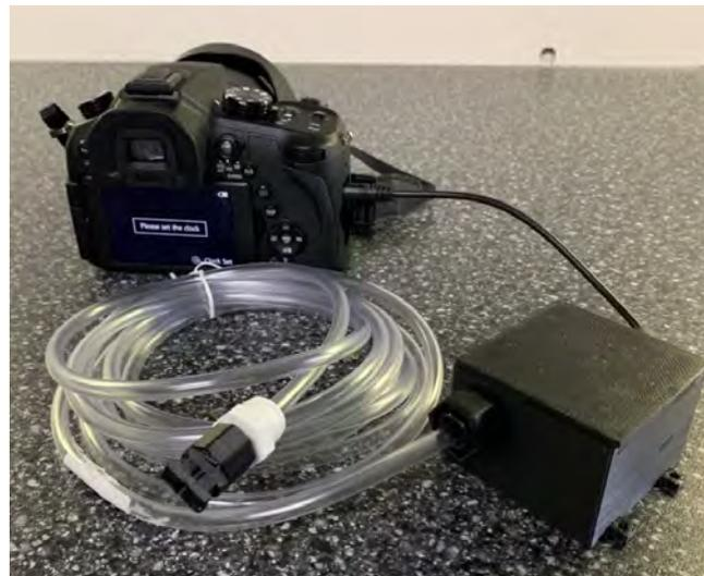
previous bite switch he had used. After interviewing both our client and sponsor, we developed target specifications based on our client's needs. Our device replaced the bite switch with a blow switch that would be more durable and less strenuous to use. The switch interfaces with the camera and triggers the shutter with a small burst of air, representing a significant improvement compared to the bite switch. Using a blow switch allows for long term use and increased comfort for our client.
