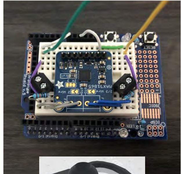
consists of an Arduino microcontroller, infrared thermometer, and 3D printed Arduino housing and earpiece. The infrared thermometer is located inside of the earpiece and focused on the tympanic membrane. The sensor sends the output to the Arduino via a wire, where the data are stored.
