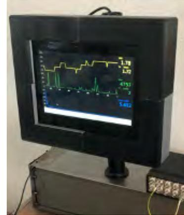
They then undergo a peak detection scheme to identify the QRS complex and systolic magnitude for the ECG and BP waveforms, respectively. This is then serially communicated to a Graphical User Interface (GUI) running on a Raspberry Pi that facilitates user interaction with the data. The GUI has various capabilities such as external data download, flagging and comment on specific data points, and trend analysis for the input HRV and BRG data.
