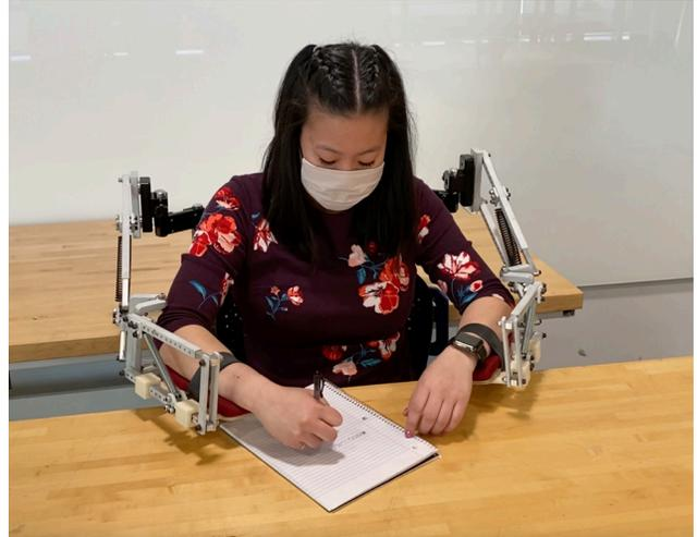
arm supports have tension springs which remove the weight of gravity from the client's arms, allowing for more independence.
