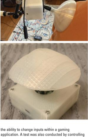
the ability to change inputs within a gaming application. A test was also conducted by controlling the device with different extremities to ensure that fine motor control was not needed to control the device effectively. While each team member was able to control the device, customer tests are planned to determine whether the device functions efficiently at this time.
