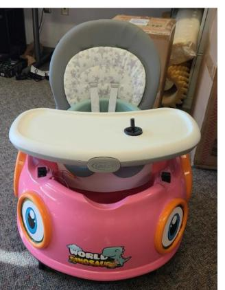
and be much lighter than earlier cars to help families more easily transport the vehicle. The vehicle will be built, wired, and programmed to respond in a manner similar to an electric-powered wheelchair with research focusing on the joystick control.
